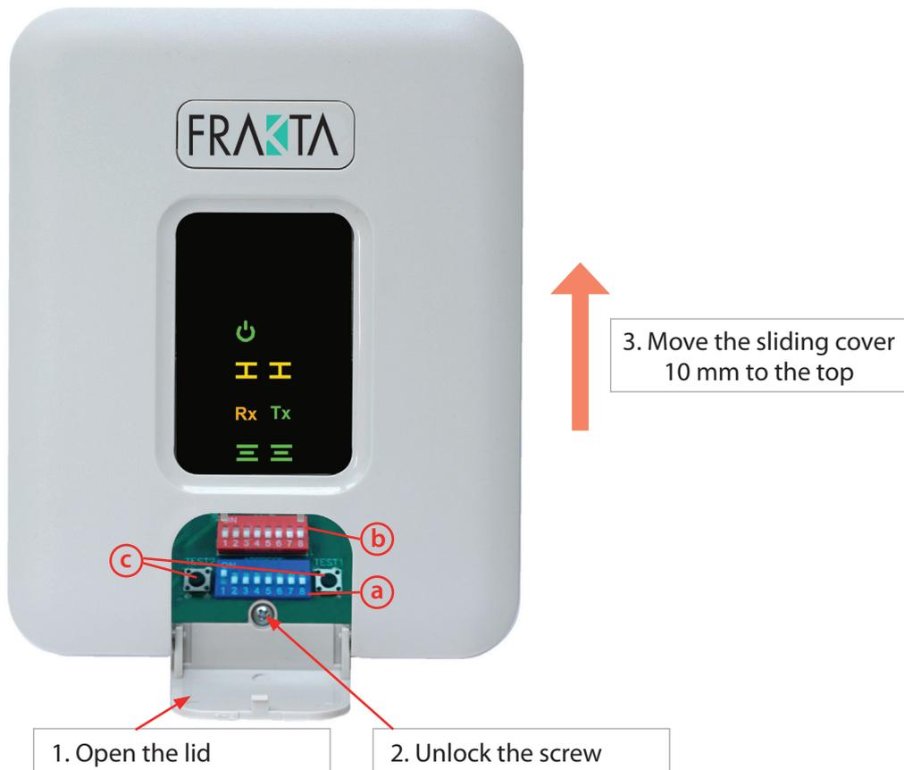
1. Open the small lid on the lower end of the housing by flapping up the cover
