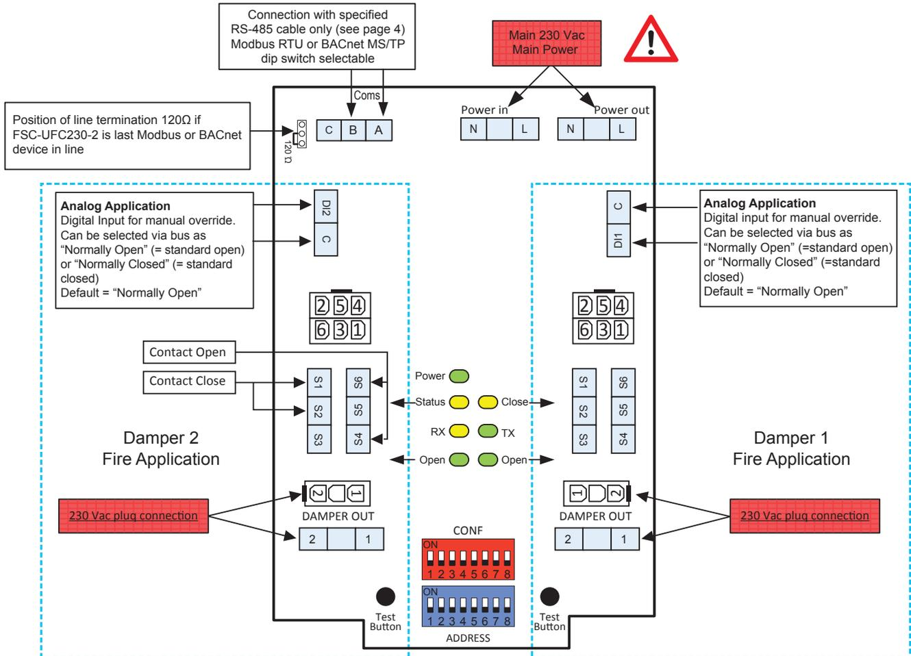
**IMPORTANT:** If only one actuator is connected to the FSC-UFC230-2 the LEDs of the side where no actuator is connected indicate an alarm. A jumper has to be installed between S4 and S6 in the terminal where there is no actuator connected, to indicate an "opened" position in the LED. If the second connection is not activated via bus, there will be no alarm signal on the bus system.
