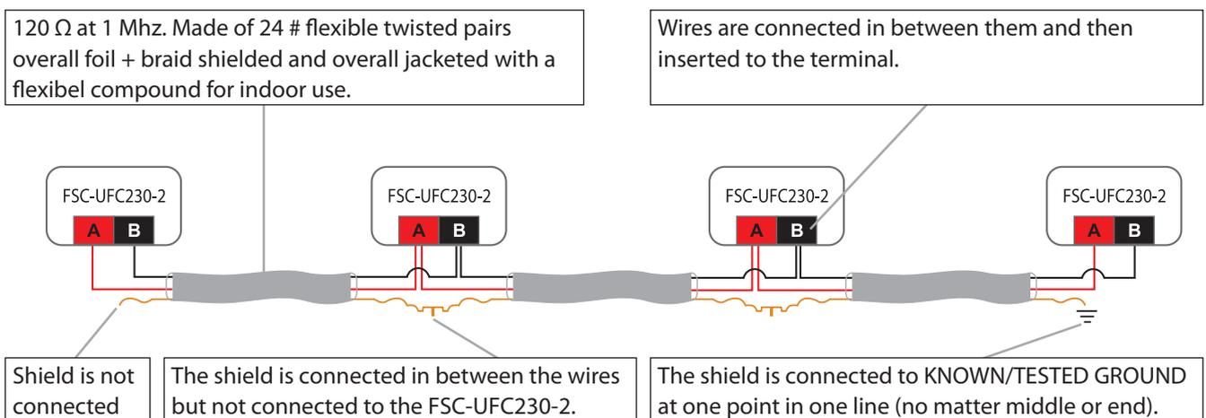
← Up to 1'200 meters and max. 100 FSC-UFC230-2 with Modbus RTU and 65 FSC-UFC230-2 with BACnet MS/TP →
